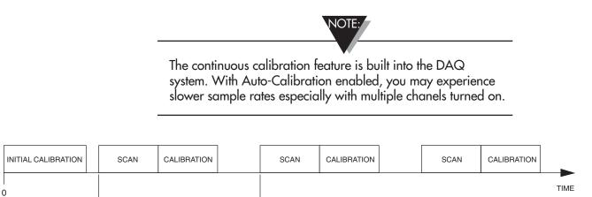
Figure 4-27. Calibration/Scan Arrangement
